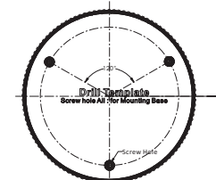
Figure 2-1 The Drill Template
